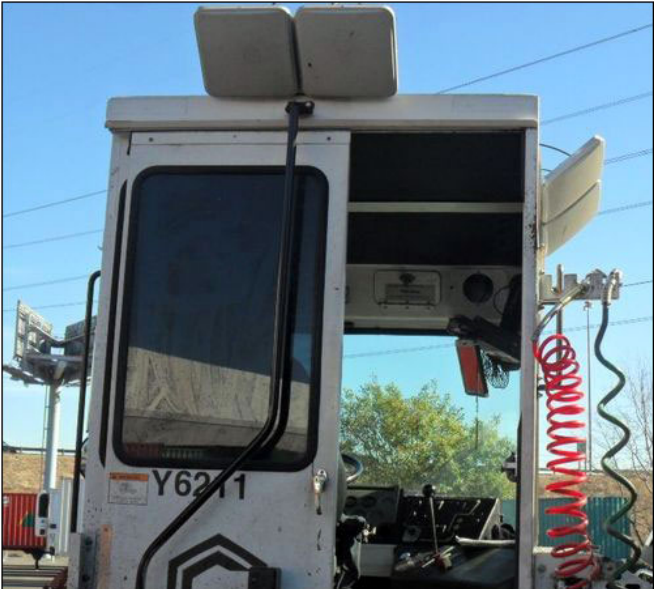
DSC Logistics' yard goat has RFID reader antennas installed on the side and back of the driver's cab.
