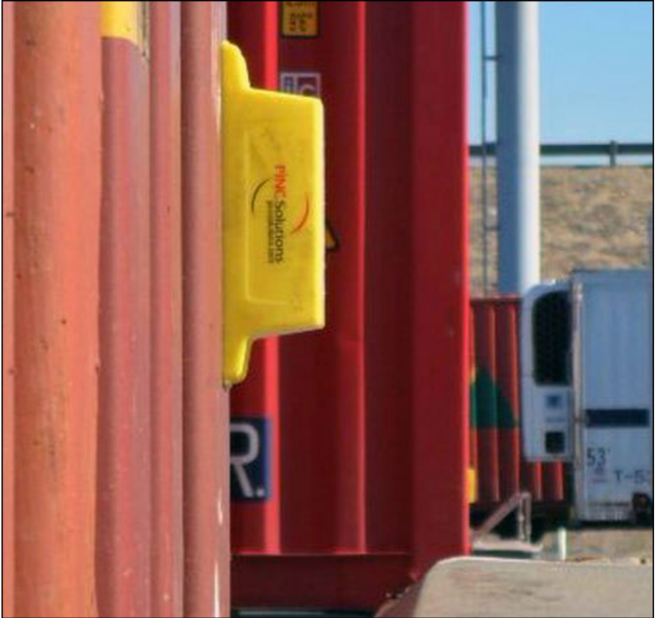
Trailers that are repeatedly stored at DSC Logistics' Mira Loma yards have an EPC Gen 2 passive RFID tag bolted to their exterior.
